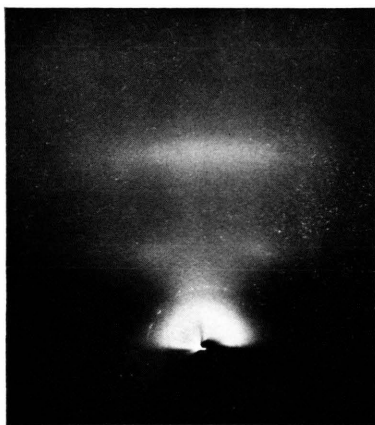
Fig. 3. Reflection electron diffraction pattern from tripalmitate of (1,2,3/0) cyclopentane-1,2,3-triol on polished brass surface.
